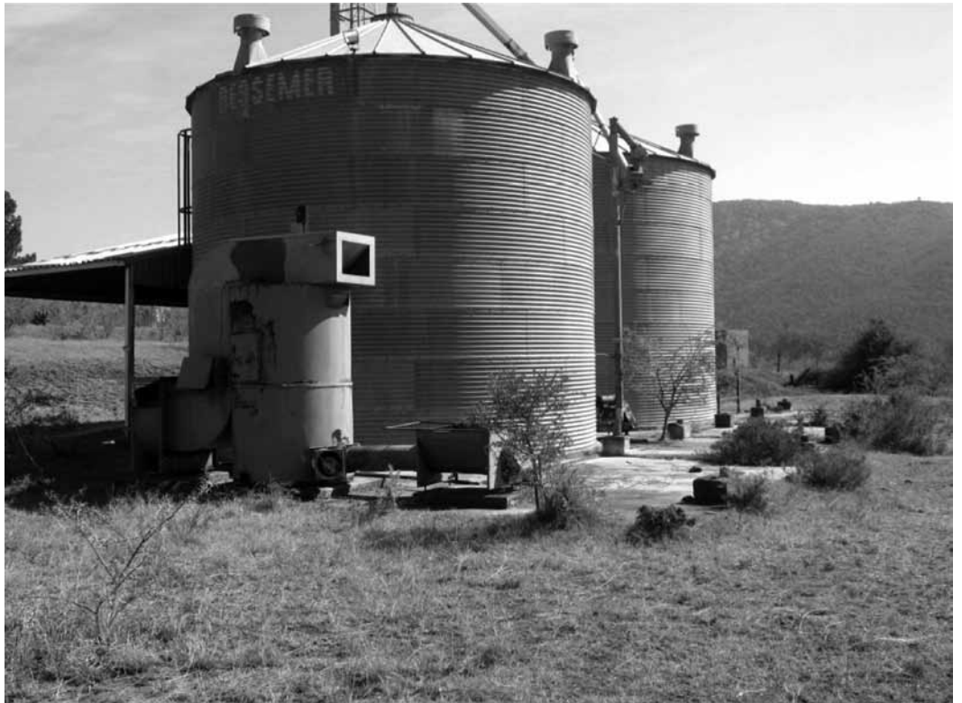
Figure 5.4: A facility used to dry maize (maize drier) at Zanyokwe Irrigation Scheme
